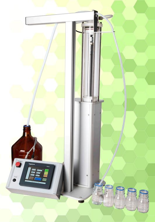
Volumetric dispenser for large flows with a programmable volume from <30 to 1100 ml.
