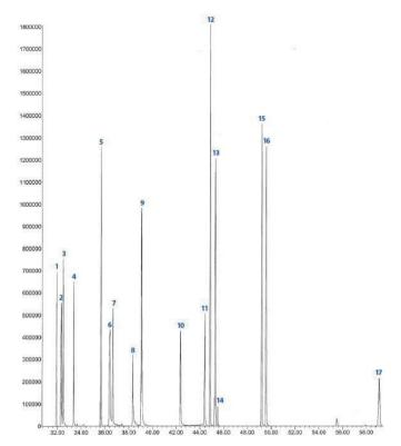
**Figure 2.** GC-MS Total Ion Chromatogram – 100 ppb Spiked Strawberry Sample. TIC displays the elution profile of the 17 pesticide standards extraction from the 100 ppb spiked strawberry sample post QuEChERs extraction.
