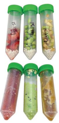
Figure 1. Produce Samples Pre and Post Homogenization. 15 g samples of strawberry, soybeans, and apples were homogenized on the Biotage<sup>®</sup> Lysera with 15 g of ceramic beads in 30 seconds.
