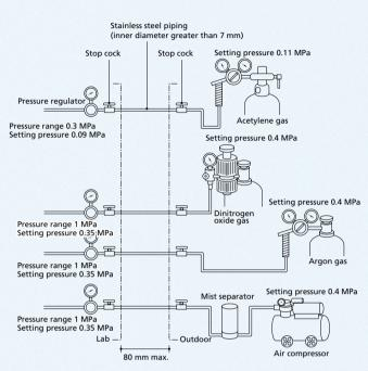
Example of recommended piping for the atomic absorption system
