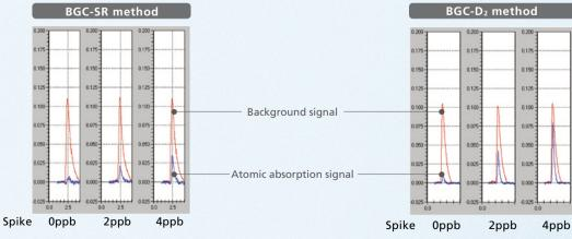
It can be seen that the sensitivity is higher with the BGC-D<sub>2</sub> method.
