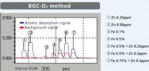
The identical 0.5 ppm Zn solution is accurately corrected to the same absorbance at (2) and (6).
