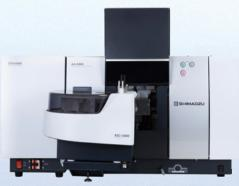
AA-6880F Dual Atomizer System (with options attached)
