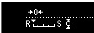
Moving it left prioritizes response and moving it right prioritizes stability. Five setting levels are available.
